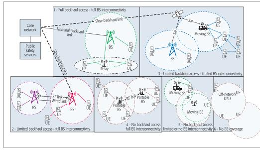
In nominal conditions, a nationwide broadband wireless PS network relies on a wired network supporting fixed wireless base stations providing planned coverage and bringing services to mobile entities relying on seamless access to the core network.
